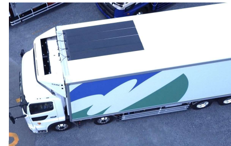
Equipped with photovoltaic power generation system
